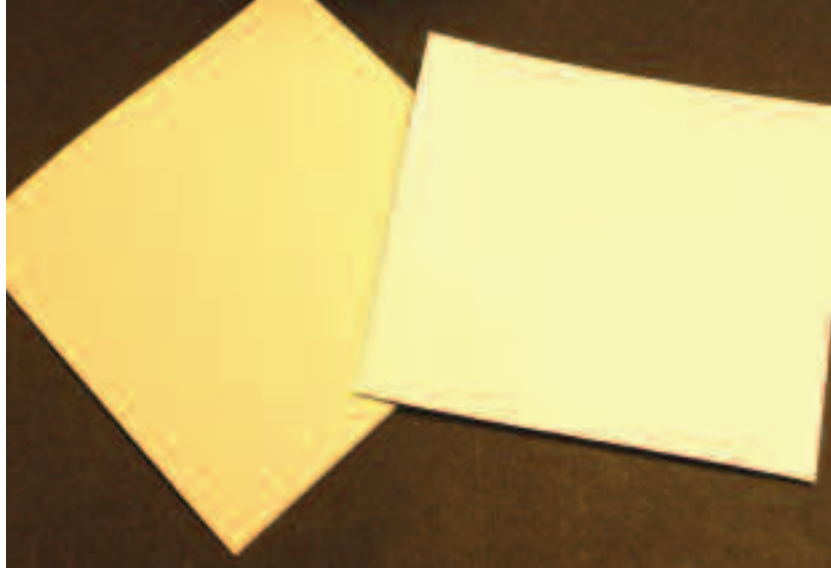
Keraflex® has two distinct surfaces prior to firing.
